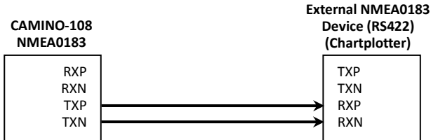
Figure 6 NMEA0183 Connection illustration
